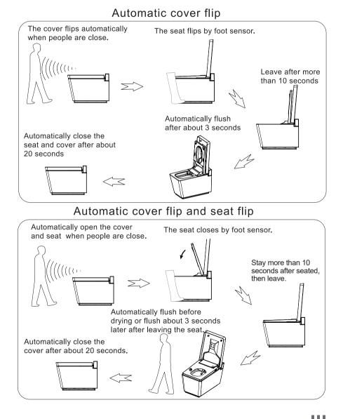
3. Automatically flush in about 3 seconds after men urinating and leaving. (only for high configurations)
